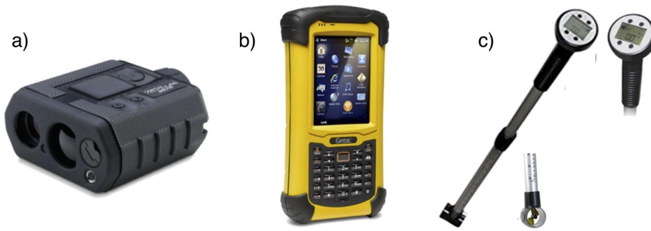
Figura 6: Telemetro laser Trupulse 360R (a), computer palmare PDA Getac PS336 (b) e correntometro Global Water Flow-Probe FP11 (c).
